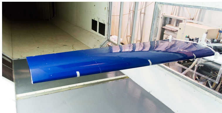
Figure 5.12: RIBES - wind tunnel model installation.
