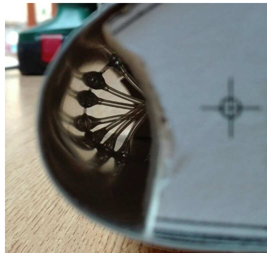
Figure A.11: RIBES - pressure taps locations.
