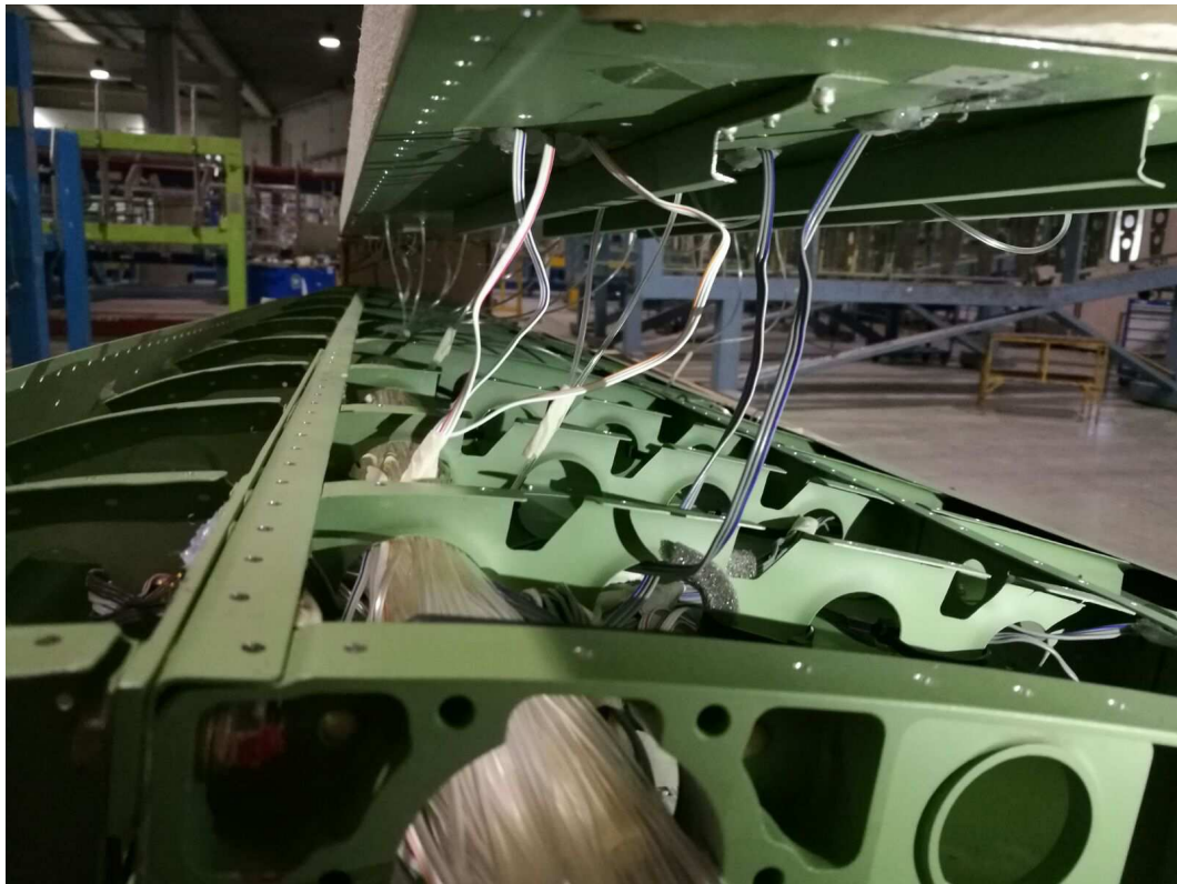
Figure A.7: RIBES - assembly of upper panel.
