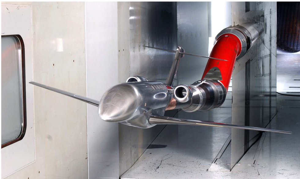
Figure 4.1: Piaggio P1XX transonic wind tunnel model (courtesy of ©Piaggio Aerospace).
